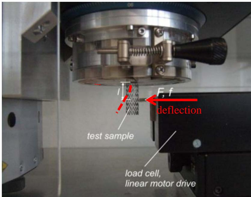
The Magmaris backbone is exposed to constant deflection and the reaction force of the scaffold backbone is measured.
