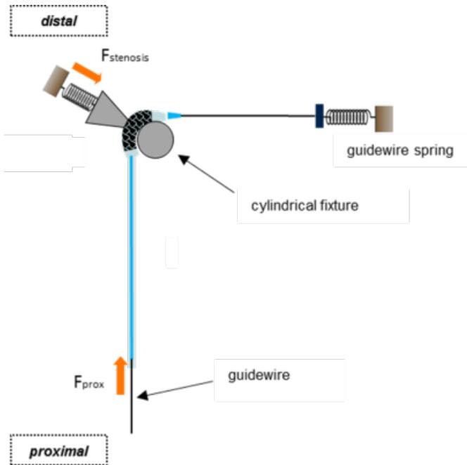
The delivery system is crossing a narrow lesion while the force is measured
