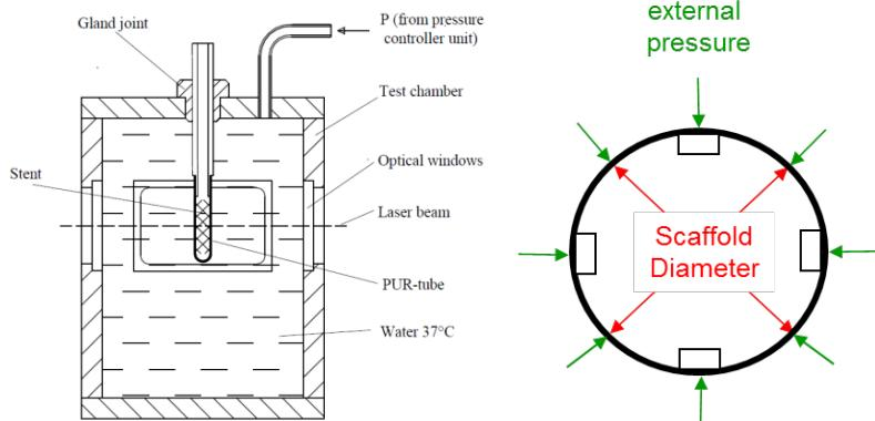
The scaffold is implanted into a thin walled tube and exposed to external pressure.
