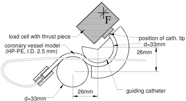
The catheter is pushed against a wall (simulating a total occlusion). The force is measured at the proximal and distal end (wall) and were expressed as a percentage by each other.
